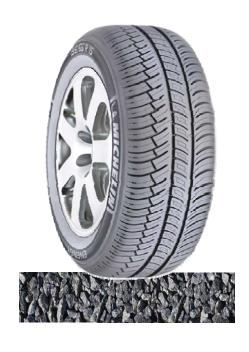
**Impacts** - At the leading edge of the tire contact patch, pavement texture and tire tread pattern induces a drumming action on the tire, and the tire responds by vibrating.
