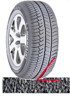
Tire – forms one half of the tire/pavement wedge in front of and behind the contact patch. The width of the tire influences the amount of magnification.
