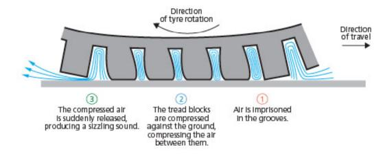
Pavement – the porosity of the pavement influences the level of the pumping action.
