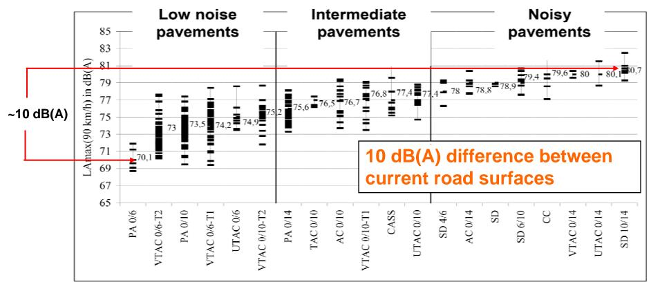
**low-noise pavements:** 0/6 and 0/10 porous asphalt (PA), 0/6 and 0/10 type 2 very thin asphalt concrete (VTAC), 0/6 ultra-thin asphalt concrete (UTAC);
