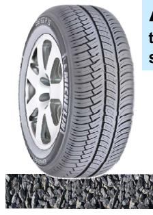
**Air pumping** — At the entrance of the contact patch, the air is imprisoned in the grooves, the compressed air is suddenly released at the exit generating noise.
